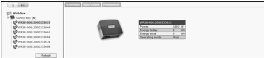
The various data pertaining to the device can be displayed and edited, if necessary, via the tabs "Overview", "Spot values" and "Parameters".
